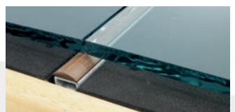
Genius RS-A can perform low emissivity (Low-E) removal operations, thanks to a series of optional devices dedicated to the various production requirements.
