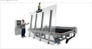
The tilting arms automatically put the glass sheet on the work
