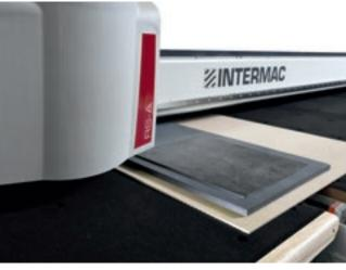
The Genius RS-A enables linear and shaped ceramic sheets to be dry-cut in a simple, intuitive manner.
